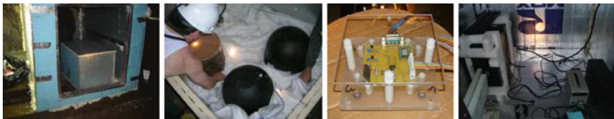
Fig. 16 Photos of the existing stations at the Homestake mine. From left to right instrument hut, seismometers, PCB operating environment monitors, and computer hut
