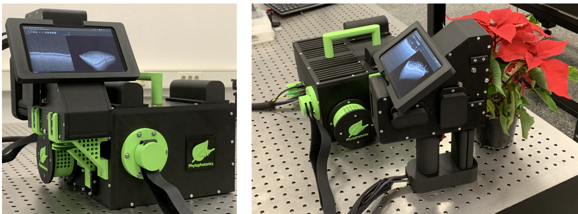
Figure 2. The portable OCT system enclosed in a 3D-printed case. Left: The handpiece is attached to the base unit for stationary use, with OCT images on the display showing a rose leaf. Right: For more flexible use, the handpiece is detached and positioned to acquire OCT images of the underside of a Euphorbia pulcherrima leaf.
