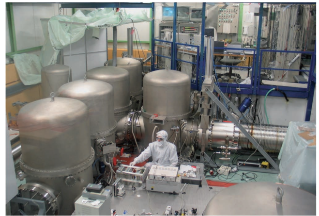
Figure 5 | GEO 600. View into the central building of the British-German GW detector located close to Hannover, Germany. The vacuum chambers contain the suspended beam splitter, power- and signal-recycling mirrors, additional input and output optics, as well as mirrors to realize a double pass of the laser light through the 600-m-long interferometer arms. Reproduced with permission from the AEI.
