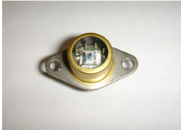
Fig. 7 Single photon detector, quantum efficiency \rho = 0.4 at 532 nm, diameter = 40 \mu\text{m}
