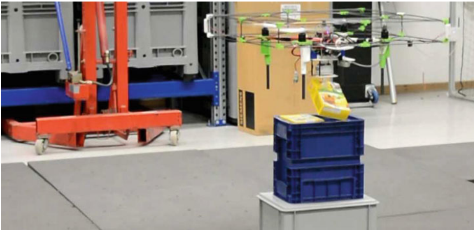
Fig. 5 In-flight grasping of a cardboard box out of a small load carrier. The box tilts to the side, as it is not grasped exactly in its center point
