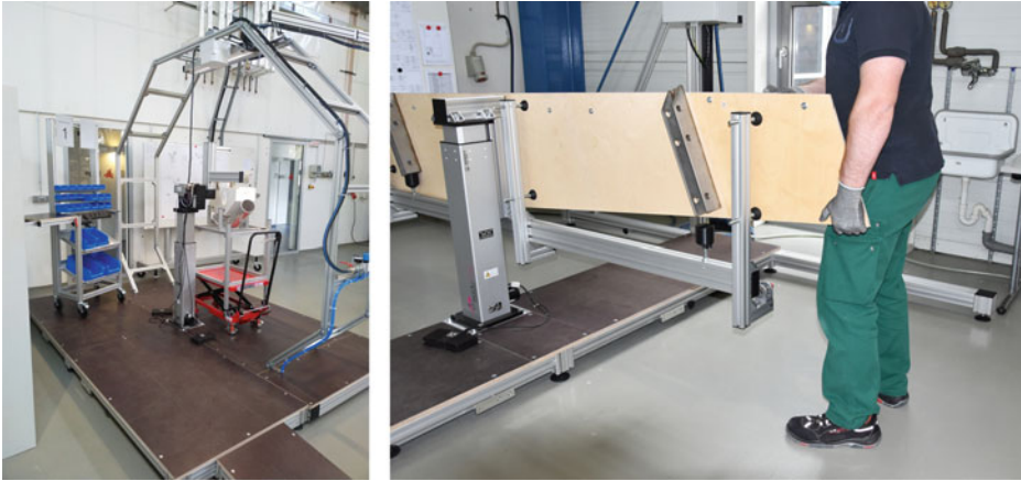
Fig. 6 Preparation for mounting support #3 to jig on mobile platform (left). Mounting of landing flap to the jig on the center platform (right)
