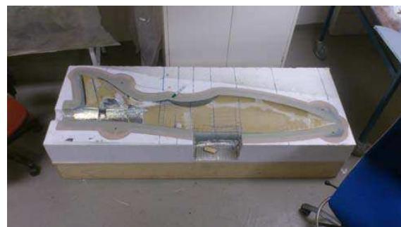
Fig. 7 Molding of the fuselage
