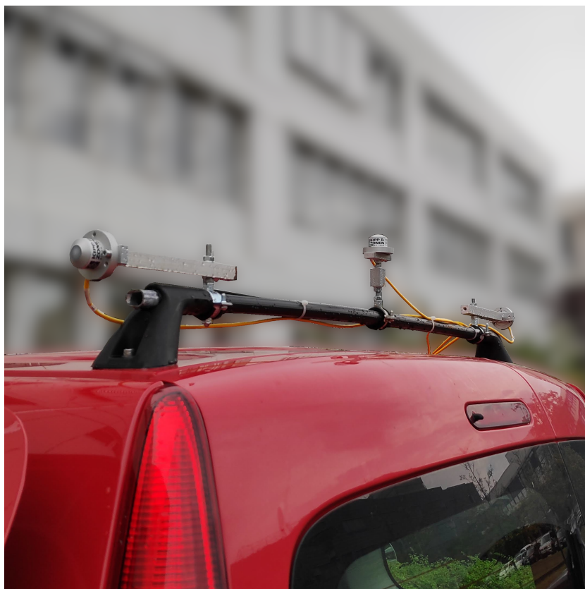
FIGURE 1 Picture of the test setup with three pyranometers mounted on the car roof. With one pyranometer looking upward and one looking to the left and to the right side each
