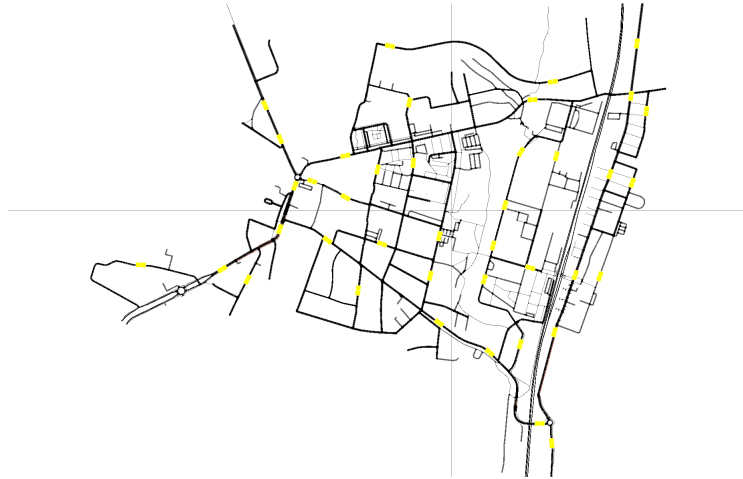
Figure 4.2: Partition of Wildau and placement of induction loop detectors.
