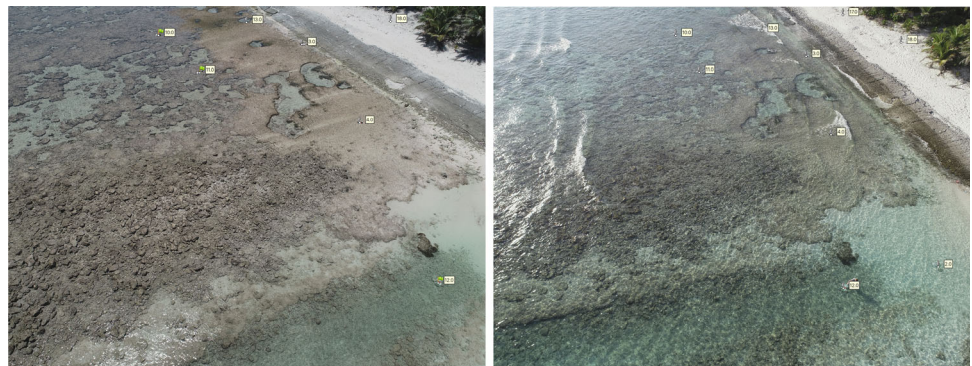
Fig. 7 Visual coastline extraction. An example of aerial images, being used to manually estimate the coastline (yellow lines) in Fig. 3. The images shown here are screenshots from METASHAPE
