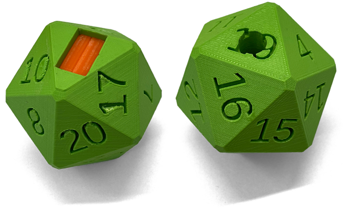
Fig. 2: The icosahedral enclosure allows the IMU to rest in 20 different orientations. It can hold the IMU case (orange) and has a hole opposite for pushing the IMU back out.
