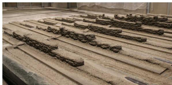
Fig. 3. Pyramidal specimen design with five layers not in scale (left) and 15 printed specimens within the machine working space (right).
