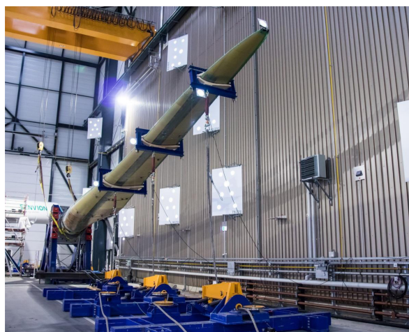
Figure 8. Photo of a static blade test configuration in flapwise direction.
