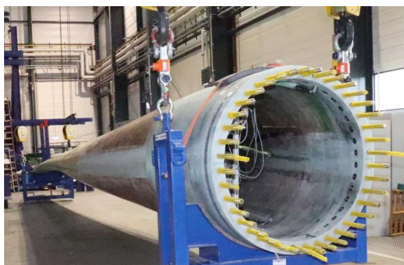
Figure 7. Setup for mass and center of gravity measurements.
