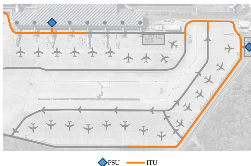
Figure 3. Exemplary dynamic inductive charging infrastructure on the apron of Cologne Bonn Airport. Source: Cologne Bonn Airport [online], 50°52′56″ N 7°07′10″ E, Height 574 m, Google Earth © GeoBasis-DE/BKG 2009, URL: http://www.google.com/earth on 29 June 2021.
