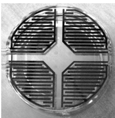
Figure 4. Face view of an electrostatic actuator for GEO 600. Four pairs of electrodes, when driven in combination, allow longitudinal, pitch and yaw adjustment of the mirror. Each actuator pad consists of two gold patterns deposited on fused silica, with a chromium intermediate layer to increase reliability. The gaps between the electrode-strips average about 4 mm.
