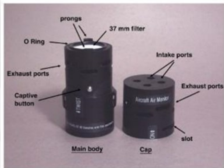
Fig. 2 - VN sampler with cap removed showing details and filter housing.
