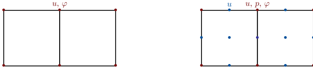
Figure 3.4: Left: conforming quadrilateral elements of the type Q_1^c Q_1^c for Chapter 4: Q_1^c for the displacement variable u and for the scalar-valued pressure variable p (red bullets). Right: conforming quadrilateral Stokes-elements of the type Q_2^c Q_1^c Q_1^c for Chapter 5: Q_2^c for the displacement components u_x and u_y (blue and red bullets) and Q_1^c for the scalar-valued pressure variable p and the phase-field function \varphi (red bullets).
