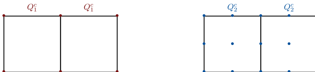
Figure 2.1: Left: conforming quadrilateral elements of the type Q_1^c defined in Equation (2.4) with four dof per cell. Right: conforming quadrilateral elements of the type Q_2^c defined in Equation (2.5) with nine dof per cell.
