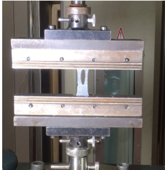
Figure 7.1: Experimental setup: punctured EPDM strip fixed via bulges on the top, and bottom boundary. The specimen has a small given notch on the left side and a (originally) circular hole. The strip is elongated on the bottom boundary until total failure.
