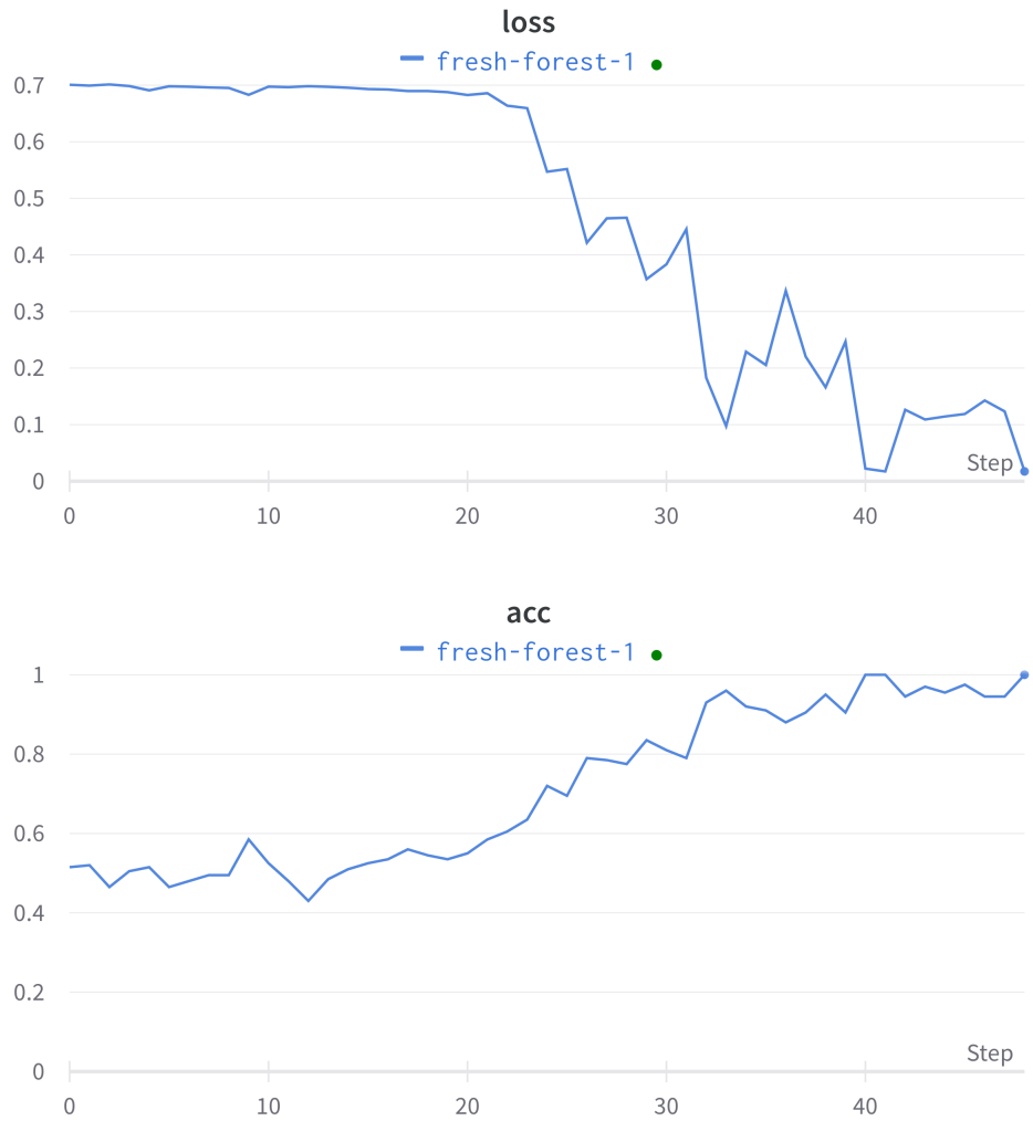
Figure 5.2: training loss and accuracy of Text CNN
