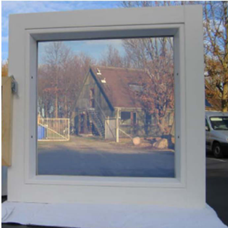
Figure 15. Super-insulating aerogel glass developed within an European project (ENK6-CT-2002-00648) for energy efficiency from[130] Reprinted with permission from Springer Science + Business Media, LLC 2006.
