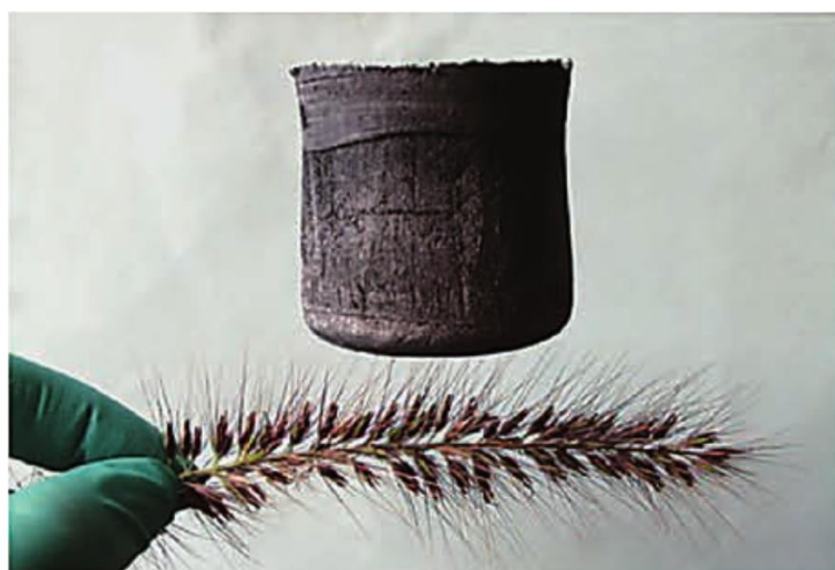
Figure 10. The currently least dense solid material known: “Ultra Flyweight Carbon Aerogel” from[86]. Reprinted with permission of Wiley-VCH.
