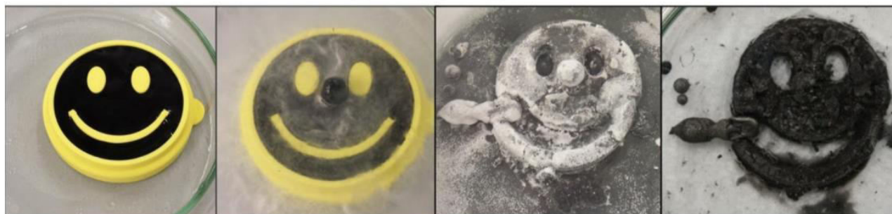
Figure SI-5.5 Shaping of the aerogels by the template approach to create a 3D smiley. (From left to right) The NP colloid is filled in a silicon mold and frozen in liquid nitrogen. While freezing due to the expansion of the water volume a “nose” is growing (note that this can happen all over the smiley). The mold is removed after freezing (where the smiley broke in the mouth area and had to be “fixed” with a “cigar”) and subsequent dried. A difficulty during the shaping is mainly the breaking apart of the shape due to the fragile nature of the aerogels.
