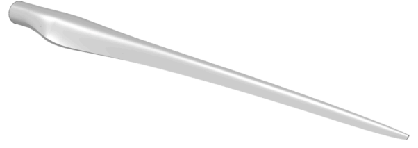
Fig. 12. CAD model of a wind turbine rotor blade.
