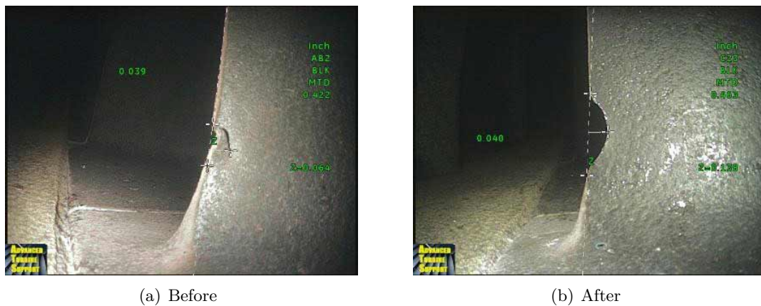
Figure 1-5: Damaged blade portion (a) before and (b) after blending. [3]
