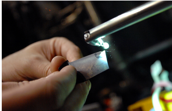
Figure 1-4: Blending tool used to manually grind down irregularities of a single compressor blade. [162]
