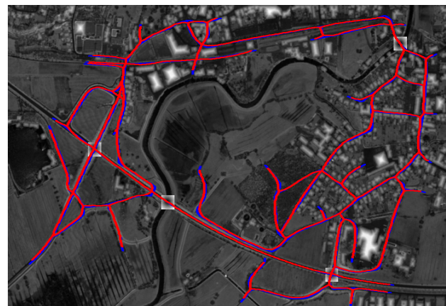
Figure 4. Adaptation of larger road networks (2199 nodes) to ALS data with bridge energy (blue: initialisation; red: final position).
