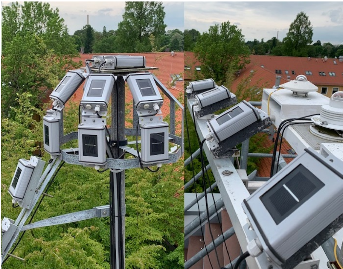
Figure 2.1: Set of silicon-based solar sensors mounted at different tilt angles and orientations, and a thermopile pyranometer available and operational at IMuK.
