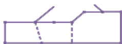
Figure 7: The operator splits the polygon at narrow parts if there is a higher order node or a concave node. An existing node is preferred if it is close to the orthogonal projection.
