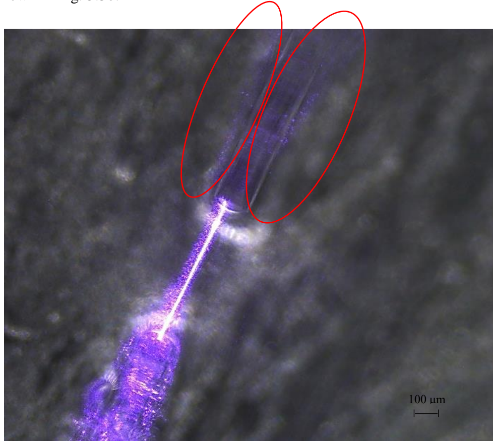
Figure 5.3b Laser beam diffraction, 1 minute after starting the curing. The amount of diffraction around the collector fiber increases constantly. However, they have not reached to the point where the PO starts decreasing
