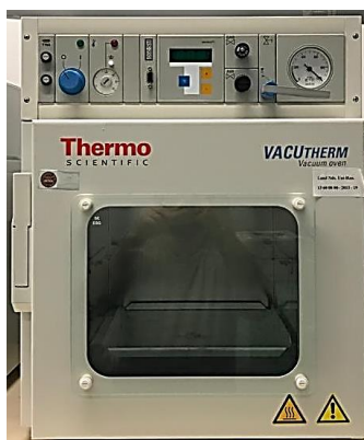
Figure 4.1 Vacuum oven using for aging. It is used to eliminate the artificial materials such as remaining air trapped inside the NOA. It is important to prevent the unwanted polymerization.
