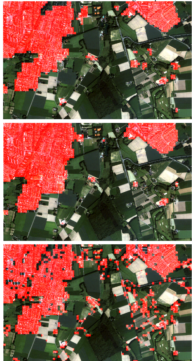
Figure 5. Test scene for s = 10 pixels. Class settlement is superimposed to the image in red. First row: ground truth; second row: CRF; third row: ML.
