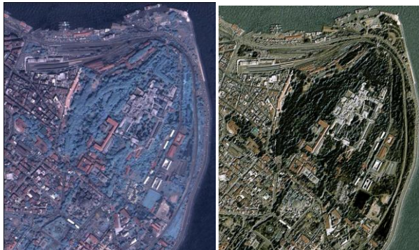
Figure 14: left: standard Brovey pan-sharpening; right: modified Brovey pan-sharpening
