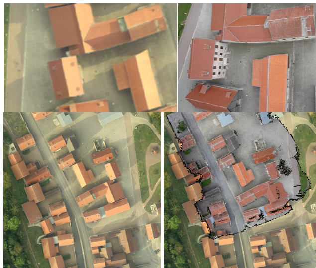
Figure 6: Top: the differences in resolution and appearance of the orthophoto (left) and a video frame (right) are enormous if the altitude of the sensor platform is low. Bottom: the workspace has been geo-referenced by registration of the synthetic image to an orthophoto.
