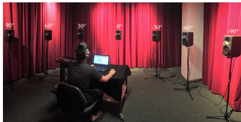
Figure 3.11: A photograph of the experimental setup. Seven loudspeakers are positioned at -90^\circ , -60^\circ , -30^\circ , 0^\circ , 30^\circ , 60^\circ , and 90^\circ relative to the subject with a distance of 1.9 m.
