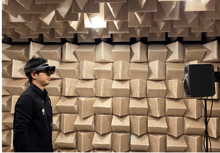
Figure 2.7: MR-based mobile 3D HRTF measurement system.
