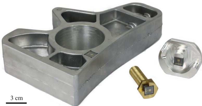
Figure 2.2 Photograph of possible application examples: sensor tag integrated in metallic parts.
