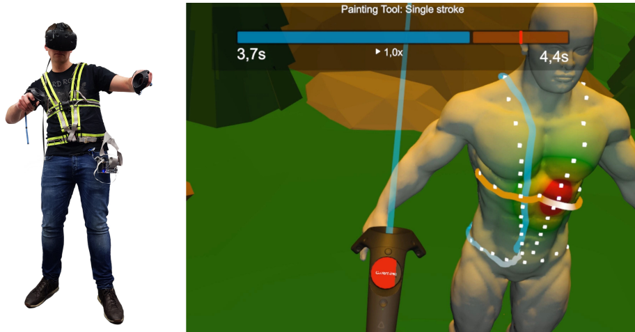
Figure 6.13.: VRTactileDraw driving the MultiWave prototype vest [187]: A wearable vibrotactile vest containing 76 actuators (left) and the user’s view inside an HTC Vive (right). The user is replaying a TP and simultaneously feels vibrations as indicated by the heatmap.
