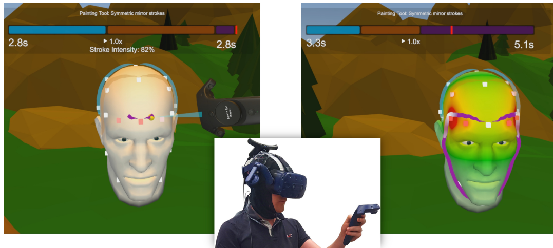
Figure 6.1.: The final version of VRTactileDraw in action. Users wear an HTC Vive Pro VR headset and a tactile user interface. A user draws symmetric strokes on the 3D model head in VR (left) and then replays the resulting pattern (right). During drawing, the user can feel the resulting tactile actuation.
