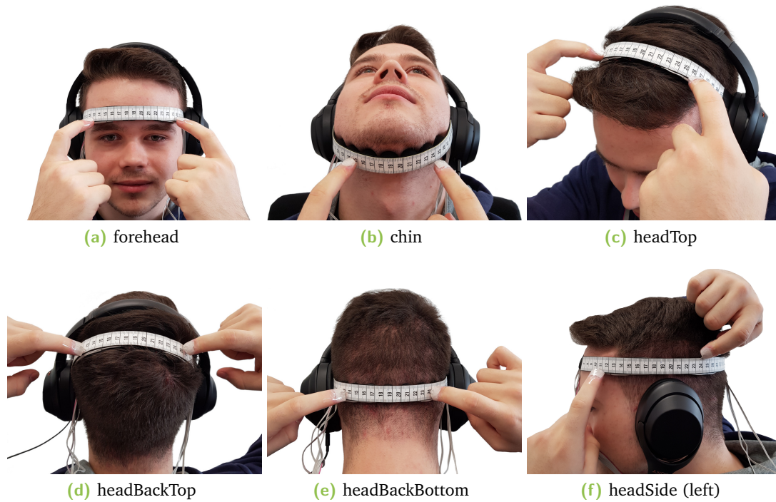
Figure 3.4.: Our prototype on different head regions for the user study. It was always attached in the same orientations, as shown in this figure for the different head regions so that the scale always went from low to high from the perspective of the experimenter to prevent reading errors.
