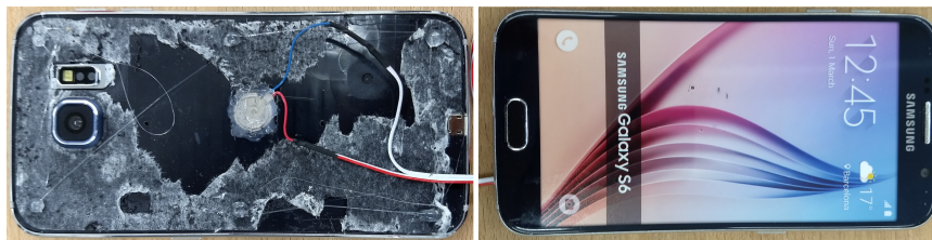
Figure 5.5.: Internal and front view of the modified Samsung Galaxy S6 dummy.
