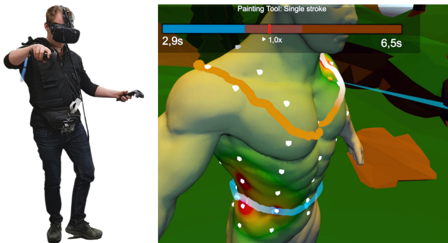
Figure 6.12.: VRTactileDraw driving a 52-actuator tactile vest mockup (left) and the users' view inside an HTC Vive (right).
