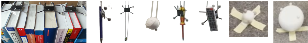
Figure 8.15.: 10 items for the Real-World 3D Guidance Experiment. From left to right (height): Three books (0.9 m), a pen (1.8 m), a Lego piece (1.1 m), a ball (1.7 m, 6 cm diameter), a screwdriver (0.8 m), a remote control (1.4 m) and two balls (3 cm and 12 cm diameter, on the ground).
