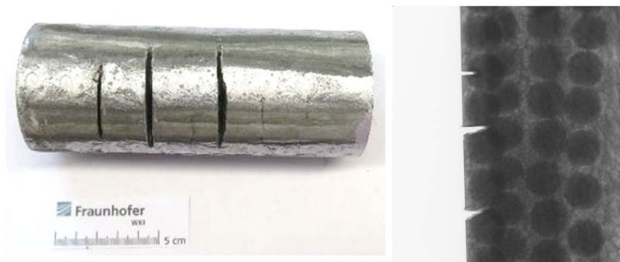
Figure 24. Cylindrical material sample after angle grinder cutting attack accompanied by an x-ray transmission image. A series of transmission images is the basis of CT measurements.
