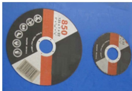
Figure 11. 125 mm cutting disc from Marcryst, before and after the cutting tests on our material. Note the massive reduction in the disc diameter from 125 mm to 40 mm (35% of the original dimension).
