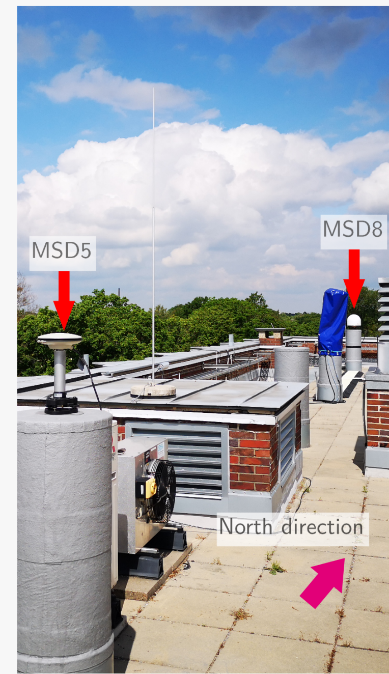
Figure 2: Combined zero / short baseline set-up with common clock for validation of the IFE-PCC patterns
