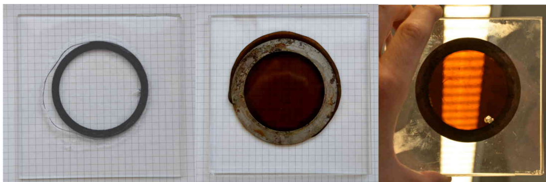
FIGURE 4.2: Photographs of PVAH layers after freezing. Left: Clear PVAH with 3 mm thick 3D printed ring. Middle: 45 mg recipe of melanin in 1 mm thick spacer ring. Right: 1 mm thick layer, prepared after 90 mg melanin recipe, held in front of ceiling lamp.
