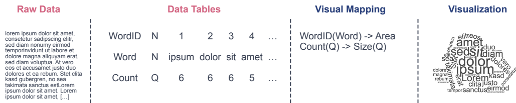
Fig. 2.2: Example of the visualization pipeline implementation for generating a wordcloud out of a text document.
