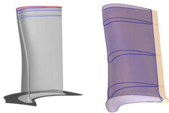
Fig. 3. (left) increase of the tip clearance; (right) loss of trailing edge material Adamczuk et al. [3])
