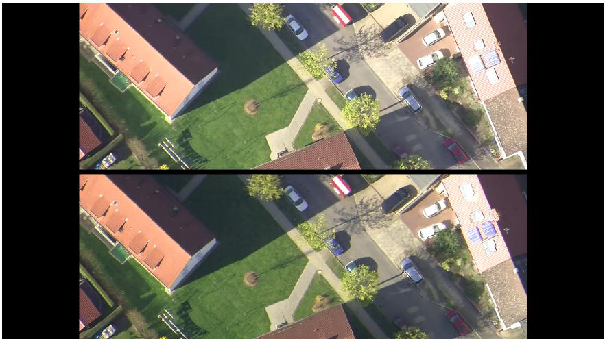
(d) 500 m sequence, best quality (top: reference, 4471 kbit/s; bottom: ROI coding, 4433 kbit/s)
