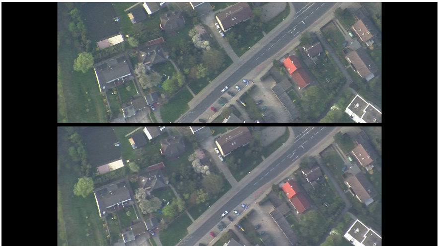
(h) 1500 m sequence, best quality (top: ROI coding, 5359 kbit/s; bottom: reference, 5296 kbit/s)
