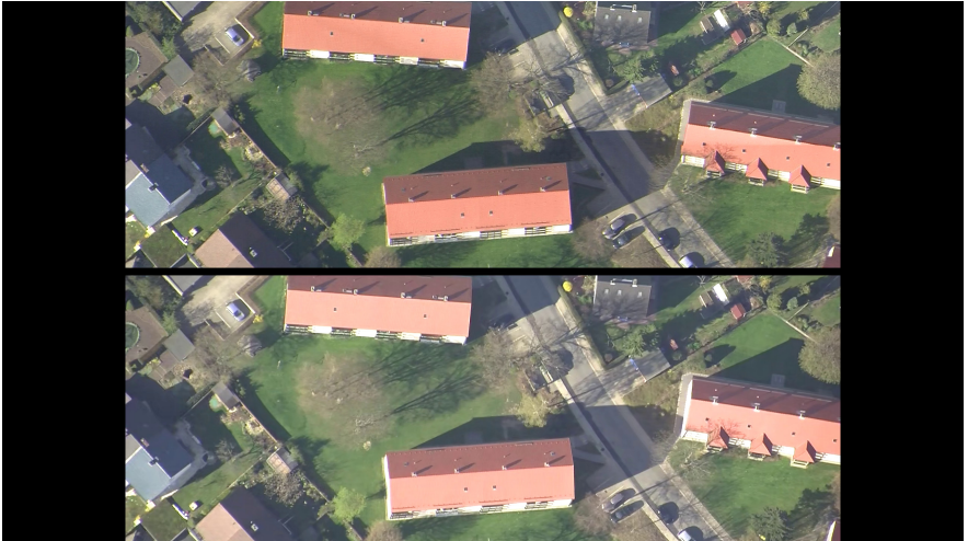
(f) 1000 m sequence, best quality (top: ROI coding, 5156 kbit/s; bottom: reference, 5243 kbit/s)
