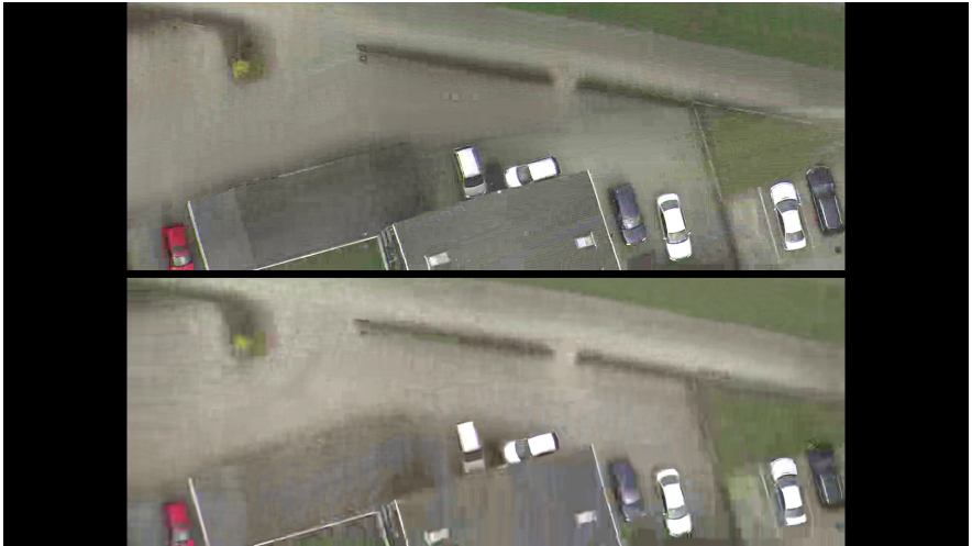
(a) 350 m sequence, worst quality (top: ROI coding, 117 kbit/s; bottom: reference, 126 kbit/s)
