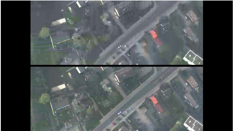
(g) 1500 m sequence, worst quality (top: reference, 105 kbit/s; bottom: ROI coding, 104 kbit/s)
