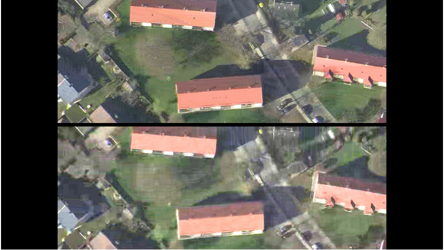
(e) 1000 m sequence, worst quality (top: ROI coding, 122 kbit/s; bottom: reference, 122 kbit/s)
