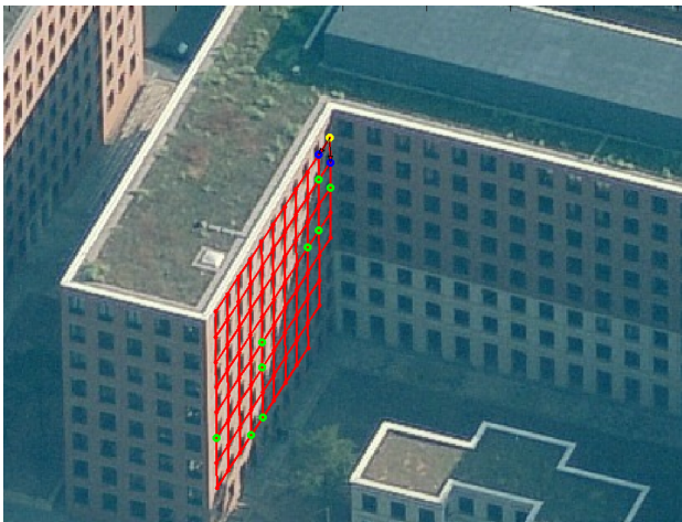
Figure 10: Lattice in oblique aerial image. Red: geocoded lattice; nodes are PS found in SAR geometry. Green: lattice positions without corresponding PS. The line of sight of the SAR sensor is roughly identical with the viewing direction of the airborne camera.
