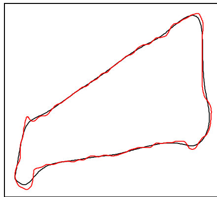
Figure 3-34: The evolved curve (red) for island 1 is approximated using cubic spline approximation technique (black) with a smoothness degree of 0.99 chosen within the range 0-1 so that the original shape is maintained.
