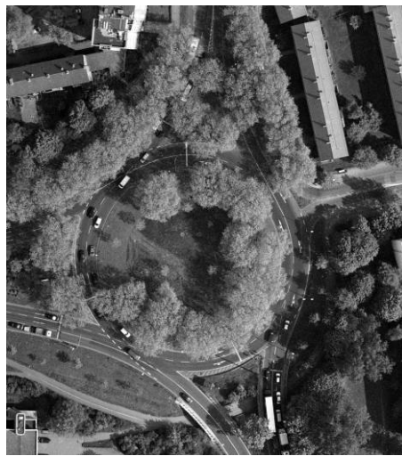
Figure 4-28: Illustrating an example in which the central island cannot be extracted due to heavy occlusions caused by trees and their shadows.
