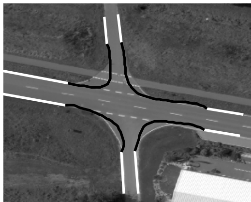
Figure 3-12 : Optimization results of the ziplock snake using tradition force field. Black curves are the result of snake optimization. White lines are the extracted road arms. Since the capture range of the external force field is small, the iterations are stopped near the initial positions.
