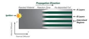
Fig. 1: schematic overview of RMS reaction
