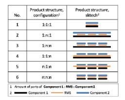
Fig. 3: Different product structures of component 1, RMS and component 2.
