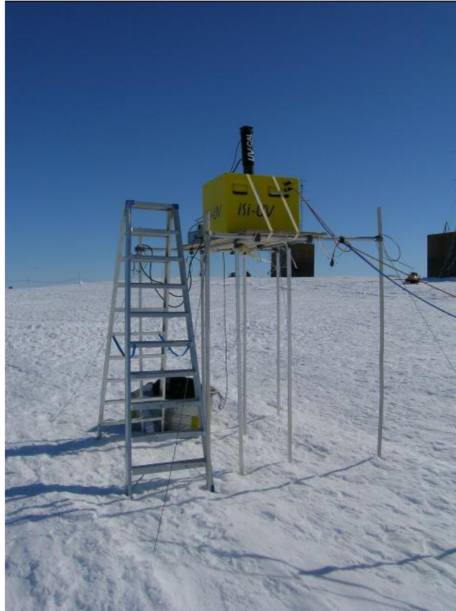
Figure 3. The AWI spectroradiometer during the process of mobile calibration.
