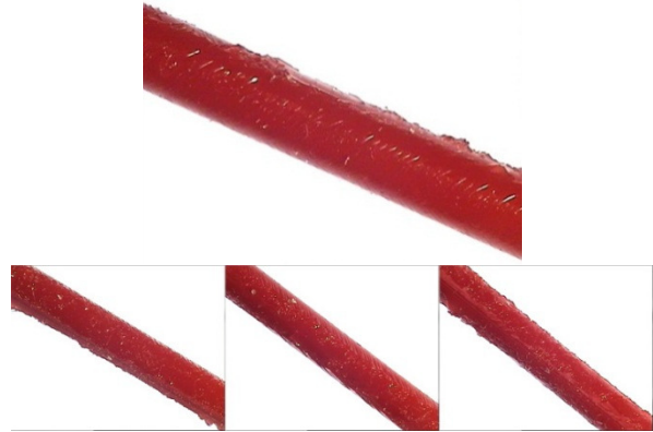
b) Inspection of damages on test specimens using microscope (200x)
