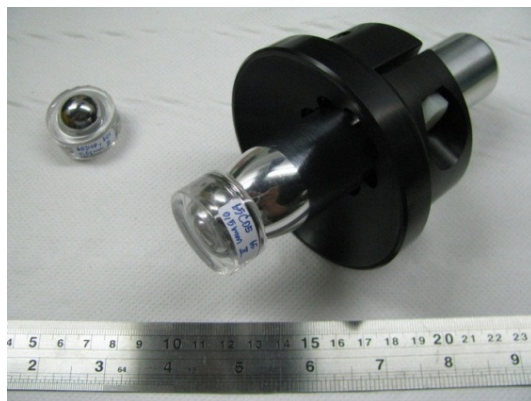
c) Installation of the test cell
