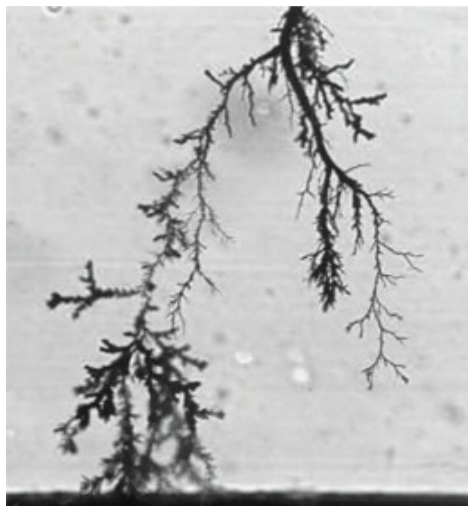
Figure 3.10: Breakdown channels in transparent polymer between point-plane electrodes
