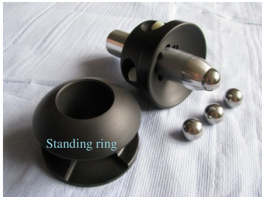
a) Test electrode and its installation
