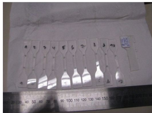
b) Specimen cured with post curing condition
