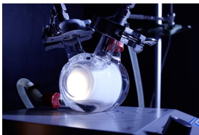
Figure 52: Quartz glass double jacket photoreactor with stainless steel flanges
