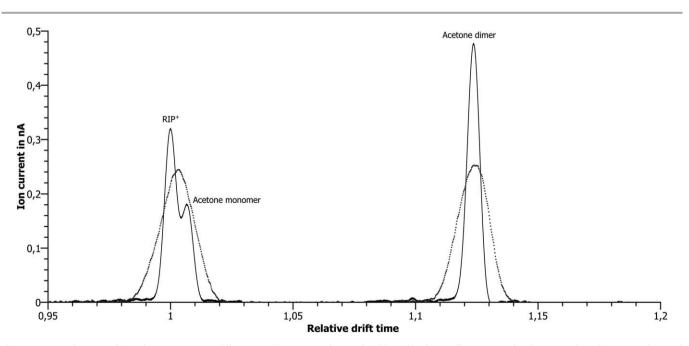
Fig. 9 Measured spectra of 20 ppb<sub>v</sub> acetone at two different resolutions. A resolution of 60 (dotted line) is insufficient to resolve the two peaks visible at a resolution of 183 (solid line).
