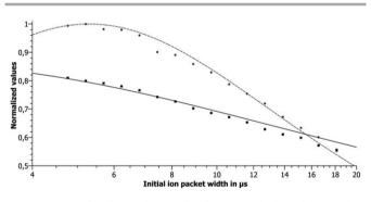
Fig. 6 Measured (dots) and calculated (lines) normalized values of the signal-tonoise-ratio (dashed line, circles) and the resolution (solid line, squares).
