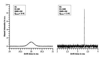
**Fig. 4** Peaks for different measurement parameters. Both panels show a 2 ms wide excerpt from the respective spectra. In (B) the initial ion packet and amplifier widths have been reduced by a factor of 27 compared to (A), and the voltage has been readjusted according to eqn (2).
