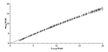
Fig. 2 Relationship between  $W_{Amp}$  and  $t_{r \ 10-90}$  obtained from a simulation. Error bars indicate standard deviation. The solid line represents a linear least-squares-fit.
