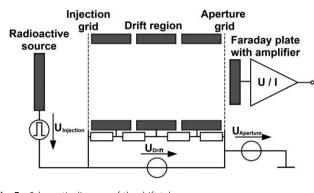
Fig. 5 Schematic diagram of the drift tube
