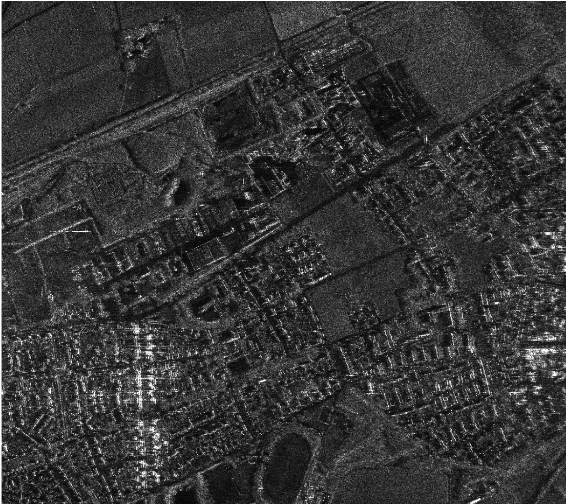
Figure 4.2.: One SAR amplitude image of the interferometric SAR image pair acquired with Intermaps AeS sensor (range direction from right to left), the image has been roughly rectified only for visualization in order to ease comparison with the optical orthophoto.
