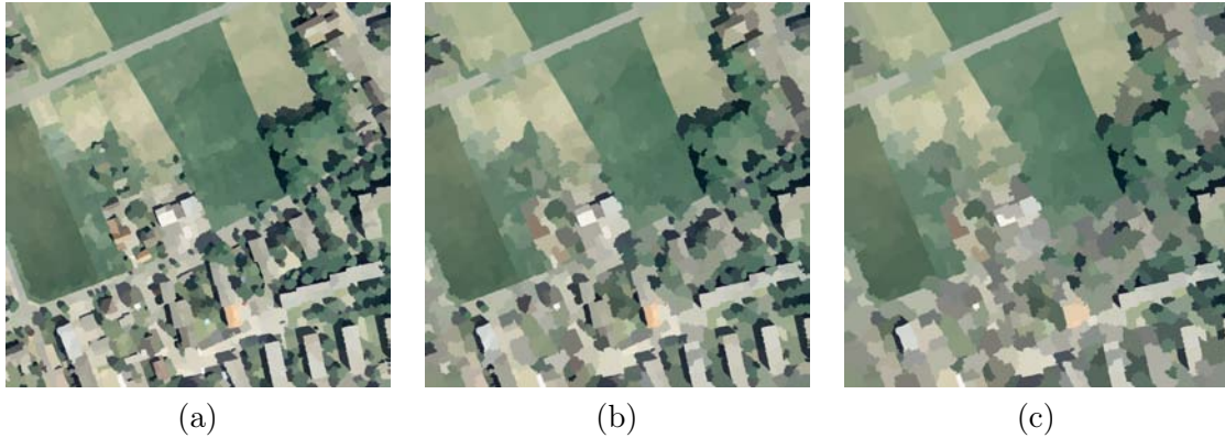
Figure 4.6.: Quickshift segmentation at three scales of the image presented in figure 4.3(a) with kernel size ks = 3 , ratio ra = 0.2 , and cuts through the tree at (a) md = 10 , (b) md = 15 , and (c) md = 18 ; its mean colour is assigned to each region.
