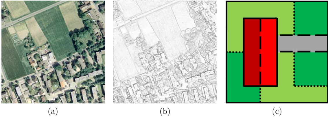
Figure 3.3.: (a) Optical aerial image, (b) gradient magnitude of its intensity channel (black: high magnitude, white: low magnitude), (c) multi-scale segmentation (three scales) into regions with gradients of three different magnitudes (solid line: coarse scale, dashed line: medium scale, dotted line: high scale).
