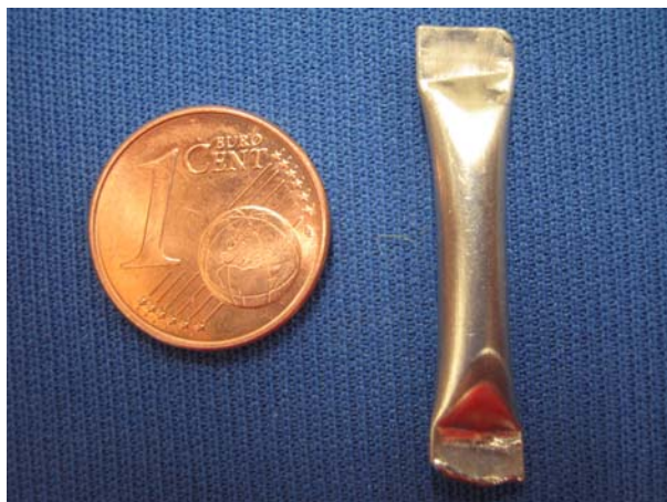
Fig. 21: Gold-palladium capsule for hydrous glass syntheses (35 mm long, 4 mm in diameter)
