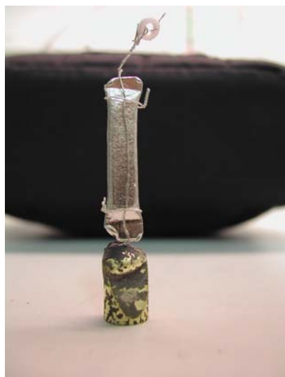
Fig.6: platinum capsule stick to the brass ramp after an experiment. The capsule is circa 3 cm long and 0.5 cm wide. After few try was clear that those long capsules were subjected to a thermal gradient during quenching, increasing their accumulated stress.
