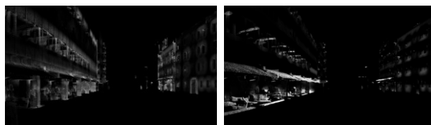
Figure 2. Image of the curvature value (left) and normal vector component in z direction (right)
