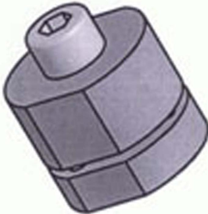
**Figure 1. Titanium clamp for mechanical induction of osteogenic differentiation.**
