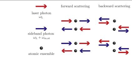
**Figure 2.** Interactions between the atomic ensemble and the light field are given by Stokes scattering processes, i.e. conversion between laser photons and sideband photons. Forward scattering processes (left column) are associated with the unmodulated spin wave  $S_0$  in equation (21). On the other side, backward scattering processes (right column) result in the two modulated spin waves  $S_{\pm 1}$  in equation (21).
