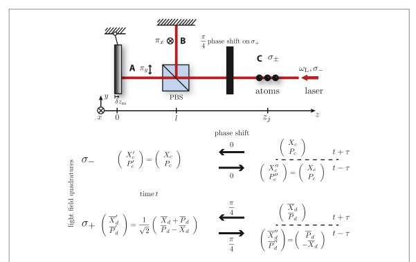
**Figure 3.** Modified setup with a phase shift on the  $\sigma_+$ -light. Below: change of quadrature basis due to the phase shift on  $\sigma_+$ -light field at different times  $t + \tau$  and t.
