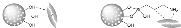
Fig 3. Scheme of the possible interactions between BDNF with (left) unmodified NPSNPs and (right) amino-modified NPSNPs. With unmodified NPSNPs, BDNF can interact via hydrogen bonds and electrostatic interactions, and with amino-modified NPSNPs via hydrogen bonding, electrostatic interactions and via hydrophobic effects. This schematic view does not show the nanoparticles, atoms and the protein with their real sizes.
