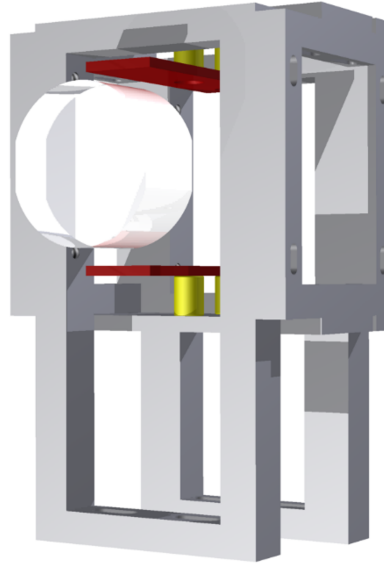
Figure 116: CAD drawing of an ESD post. The design fulfills the requirements itemized above. The structure is made from aluminum. The yellow cylinders, which separate the capacitor plates (red) from the post, are commercial ceramic insulators. The mechanical resonances of this system are shown in figure 117.
