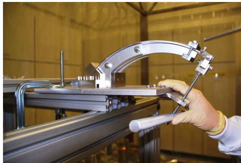
Figure 124: An additional clamp fixes the blade to the jig.
