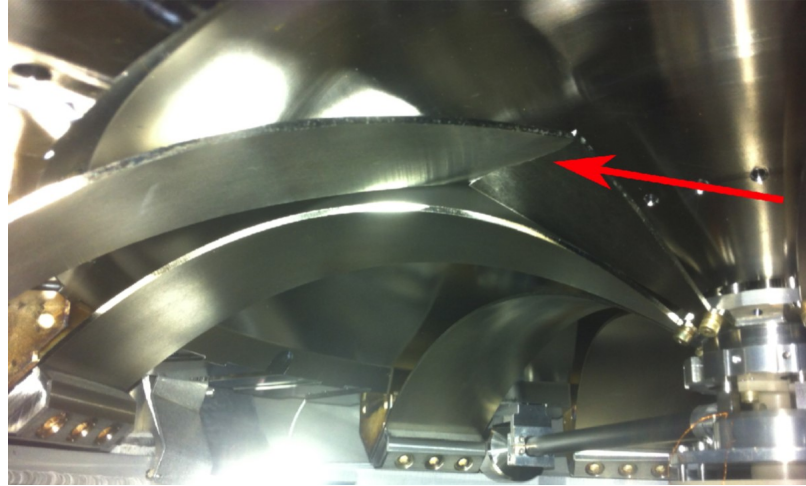
Figure 52: Photograph of a blade failure (indicated by the red arrow) in the intermediate filter of Advanced Virgo's SPRB MultiSAS. This figure is taken from [139].
