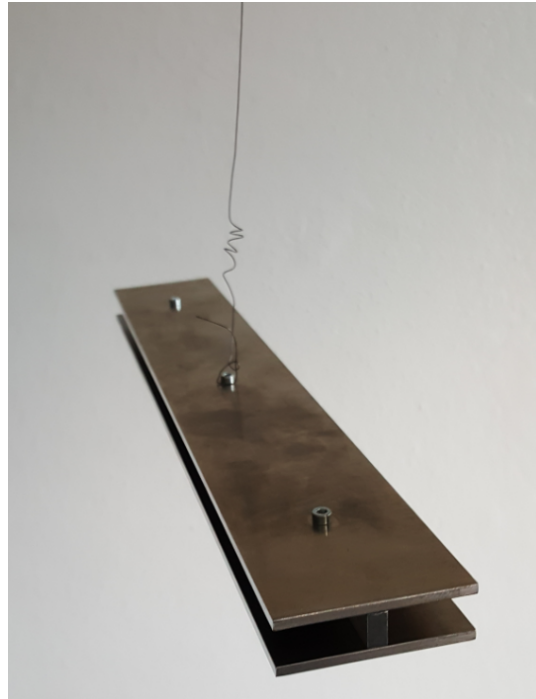
Figure 82: Experimental setup to measure the resonance frequencies. The I-beam was suspended in its center from a steel wire. In order to reduce the vertical stiffness of the wire, and therefore its influence on the structure's resonance frequencies, it was curled. The modes were excited by tapping the edges of the structure. The beam's vibration was measured with a microphone.
