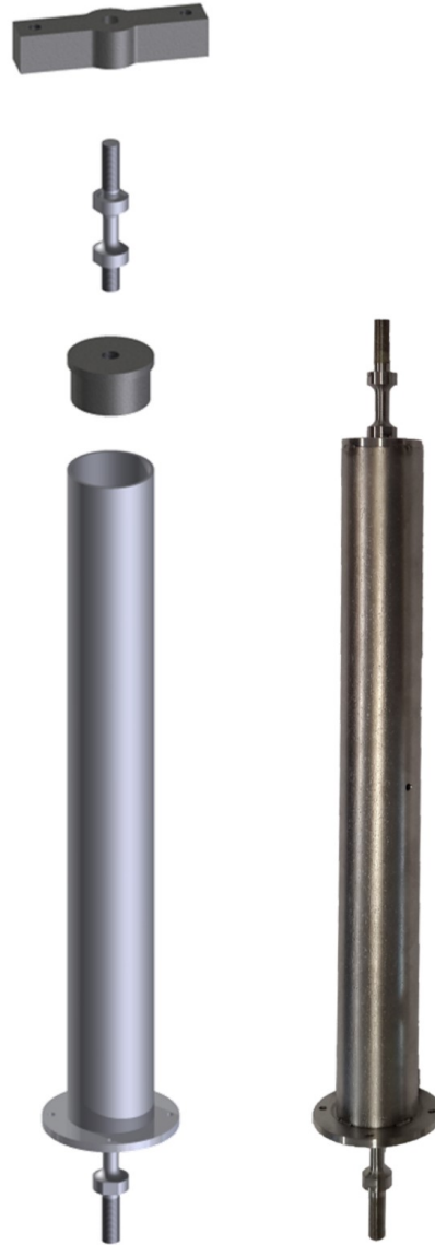
Figure 71: Mechanical design and photograph of the symmetric IP-leg. The new IP-leg consists of an identical upper and lower flexure made from titanium grade 5 and a stainless steel leg. An upper and a lower cap are welded to the stainless steel tube with 2 mm wall thickness. The bottom cap features a rim on which the original CoP tuning structure can be installed. The hole in the steel tube, visible in the photograph, is for venting the structure during the evacuation of the vacuum system.
