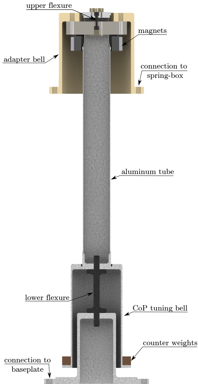
Figure 44: Section view of a single IP-leg. The whole leg is placed on a foot, which is the connection to the AEI-SAS baseplate. The dumbbell-shaped lower flexure is bolted on its lower end to the foot and on its upper end to the bottom of the leg. The leg itself is an aluminum tube with 1 mm wall thickness. The upper flexure is suspended from a stainless steel cap on the upper end of the aluminum tube. It is a 25 mm long and 3 mm thick maraging steel cylinder with a nail head on the top and the bottom for connecting it to the neighboring parts. The whole payload and the spring-box are suspended from those three upper flexures. The upper spring-box plate is resting on the rim of the upper bell. This bell is supported by a stainless steel bar which is reaching through two windows in the aluminum tube and is suspended from the upper flexure. The upper bell serves the purpose of reducing the total height of the AEI-SAS. The lower end of the IP-leg is surrounded by the lower bell. This structure is used to tune the CoP of the IP-legs. That is achieved, by loading it with counter weights.
