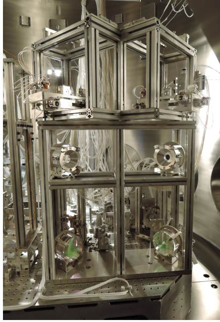
Figure 16: Photograph of frequency reference cavity suspension system for the two central table mirrors.
