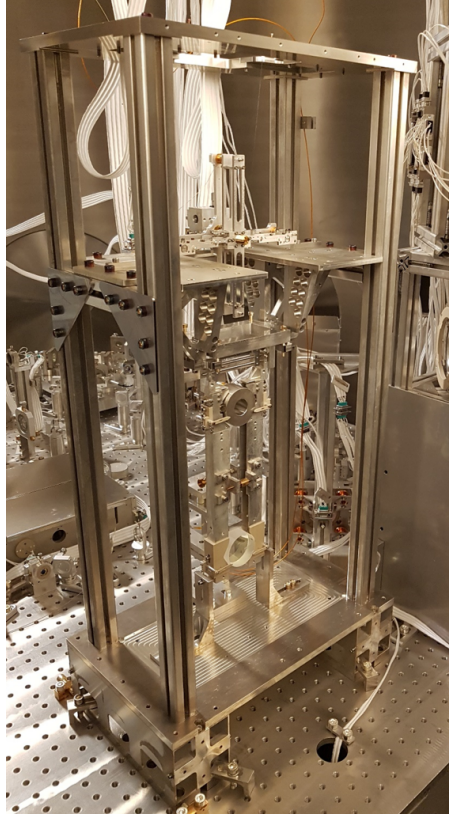
Figure 15: Photograph of the ITM suspension. The mirror is suspended as a three stage pendulum with ultimately three vertical stages. The figure shows the suspension setup for the single arm test. In the final SQL interferometer version the lower stage (intermediate mass to test mass) will be replaced by a monolithic stage.
