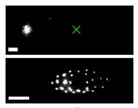
Figure 1. Top: A single Ar<sup>13+</sup> ion (position marked by cross) sympathetically cooled by a single lasercooled Be<sup>+</sup> ion. White scale bar denotes 20 µm. Bottom: A single Ar<sup>13+</sup> ion sympathetically cooled by several  $Be^+$  ions. White scale bar denotes 100  $\mu$ m.
